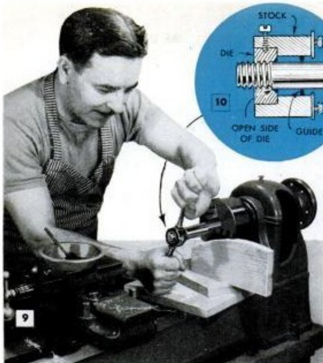
Threading with a round die held in a stock can be done in a lathe. Stock and die are reversed when threading to shoulder
