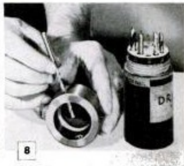
Lacking other means, determine size of internal thread with tap drill
