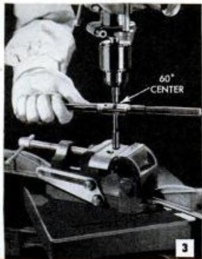
1 Ideal setup for tapping can be made on drill press. Tap is turned by hand, by pulling on belt or by using tap wrench
