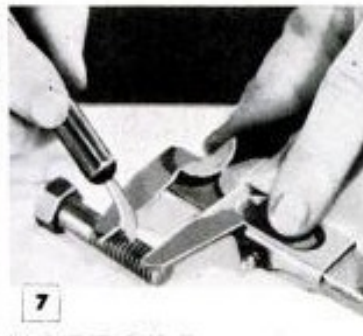
Without a pitch gauge, count the threads per inch or half inch
