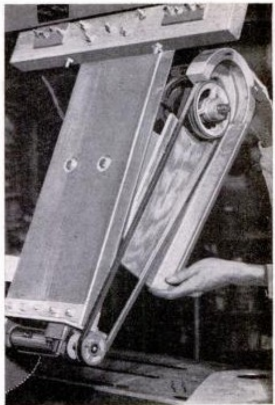
Belt guard is built up as a unit before attaching to swinging column. Note relative size of pulleys
