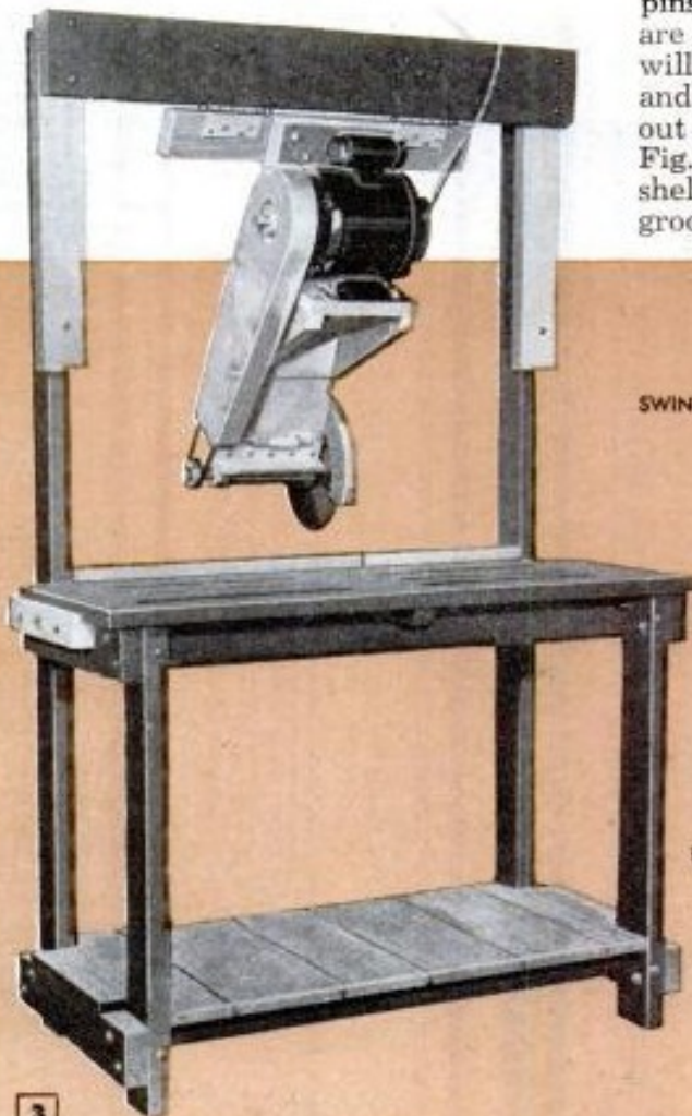
By using angle blocks clamped against the fence, you can make angle cuts up to 45 deg. on narrow stock
