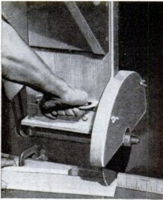
By using angle blocks clamped against the fence, you can make angle cuts up to 45 deg. on narrow stock
