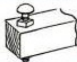
11 DRILLING holes for seams is done easily with work supported on bolt fitted in end of wooden block clamped to the drill-press table
