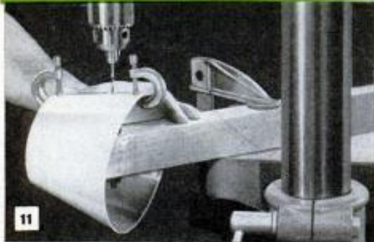
11 DRILLING holes for seams is done easily with work supported on bolt fitted in end of wooden block clamped to the drill-press table
