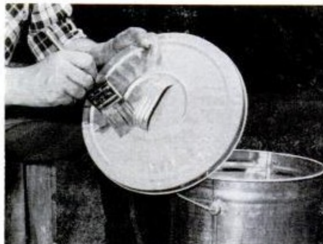
ON REFUSE CANS to double their life. You can make them more sightly, too, with just a primer coat. Or add a top coat of house paint.
