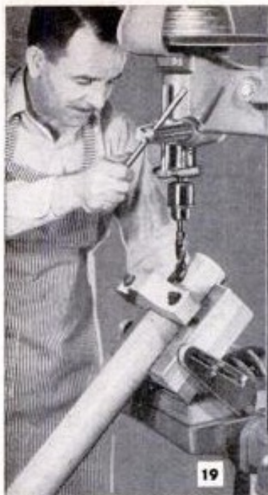
MOUNTING THE WORK CAN BE DONE BY ANY OF THE THREE METHODS SHOWN ABOVE. THE ANGLE VISE DETAILED AT THE RIGHT AND SHOWN IN USE IN THE LEFT-HAND PHOTO ABOVE, IS USEFUL FOR A VARIETY OF DIFFERENT JOBS
