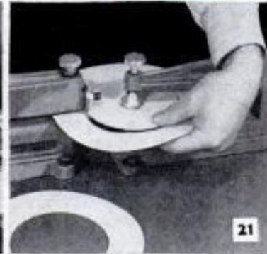
Circles are cut by using a pivot, which is an accessory to the shear. Cut may be started at edge of work, as in bandsawing, or top cutter can be forced through work at any point. To prevent distortion, inside cuts are made with minimum overlap of the cutters. On outside cuts, snip away the waste as cut progresses
