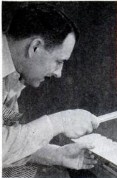
Hand-operated punch makes clean, round holes for rivets or decorative effects. Square dies are available for certain type punches, also accessory shear blades in various sizes
