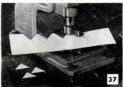
Above, cutting in from edge with shear. Below, notching edge with shear blade
