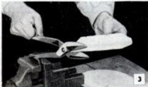
Snips should be held square with work, except aviation type which cut best with right tilt. Below, vise mounting aids in cutting thick stock
