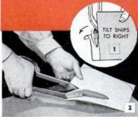
Snips should be held square with work, except aviation type which cut best with right tilt. Below, vise mounting aids in cutting thick stock
