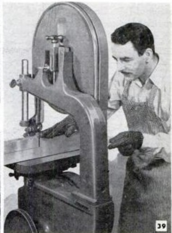
Bandsaw used as friction saw cuts fast and accurately on sheet metals of all kinds up to \frac{1}{8} in. thickness
