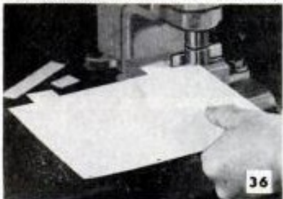
Above, cutting in from edge with shear. Below, notching edge with shear blade
