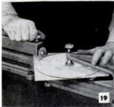
Circles are cut by using a pivot, which is an accessory to the shear. Cut may be started at edge of work, as in bandsawing, or top cutter can be forced through work at any point. To prevent distortion, inside cuts are made with minimum overlap of the cutters. On outside cuts, snip away the waste as cut progresses
